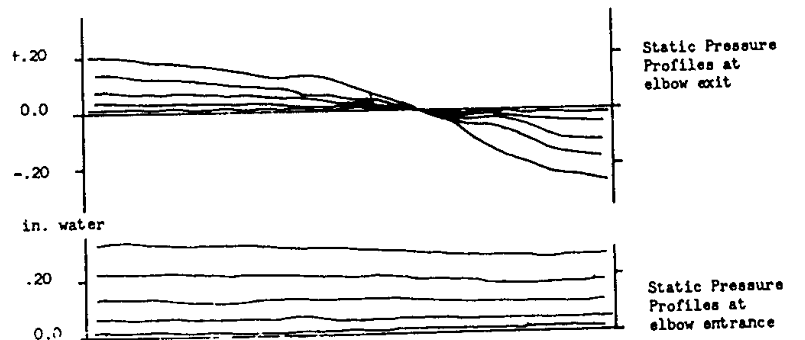
Fig. 10 Static pressure and velocity profiles for 2" radius single thickness vanes spaced 1.5"
